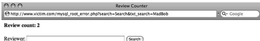
Figure 5.6 Query for “MadBob” Returning a Count of Two Reviews, Used As TRUE Inference
