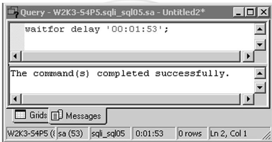
Figure 5.5 Executing WAITFOR DELAY
