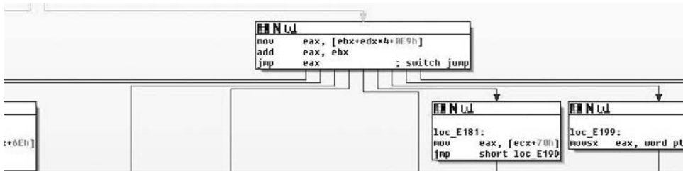
Figure 6-4: After you run the script, IDA Pro finds all the possible jump destinations for this switch statement.
