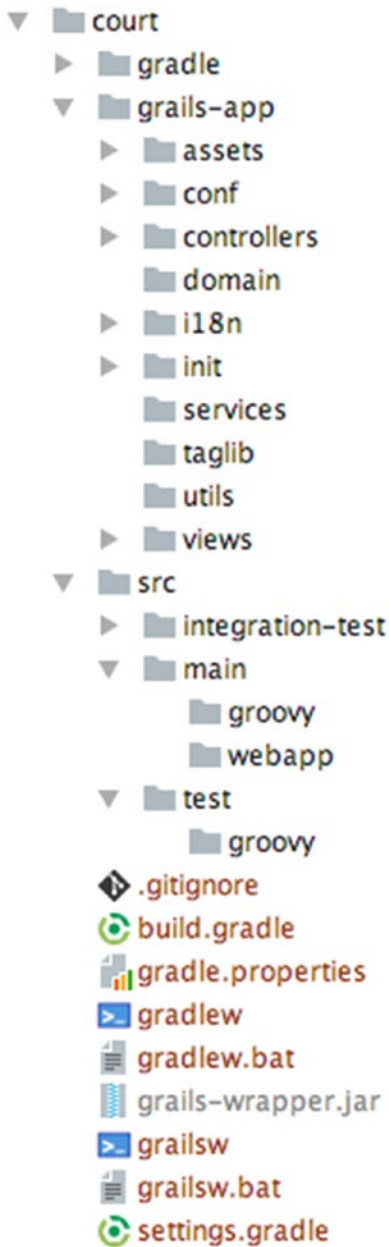
Figure 17-1. Grails application project structure
