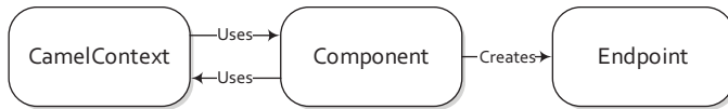
Figure 7.1 A component creates endpoints and may use the CamelContext’s facilities to accomplish this.
