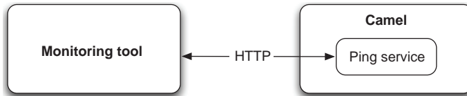
Figure 12.1 A monitoring tool monitors Camel with a ping service by sending periodic HTTP GET requests.
